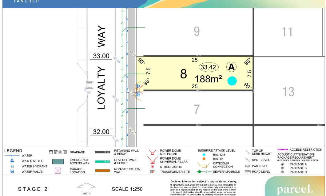
All retaining walls and associated easements are shown
